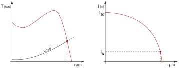
For an individual compressor, the normal starting current ISC will be 4-5 times its rated current IN. If the unit is equipped with the electronic soft-starter accessory, the starting of each compressor is done with an acceleration ramp that allows the effective value (rms value) of the inrush current of the individual compressor to be lowered.
