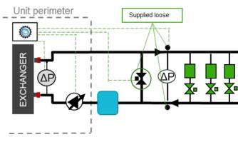
Bluethink solution for a variable flow rate system, consisting solely of a user-side primary circuit. Flowzer VFPP includes:
