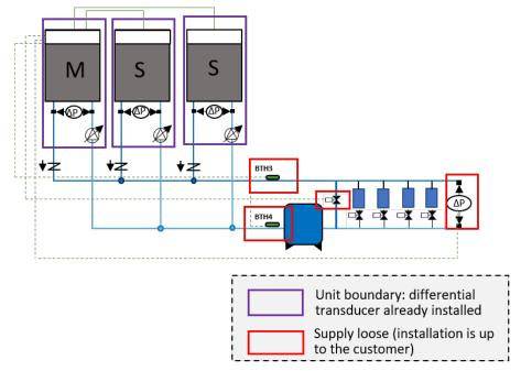
It is obligatory for the option to be combined with the Flowzer VP (inverter) and with one of the hydraulic modules that can be selected for the unit.
