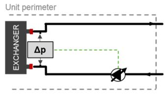
Flowzer VDE requires a differential pressure transducer to be installed in the machine. Through this transducer, the inverter can gauge the actual pressure at the ends of the heat exchanger installed in the machine and it can automatically adapt the pump speed for a constant flow value under all conditions. Flowzer VDE must be combined with Flowzer VP.
