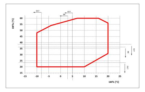
**LWTs:** water outlet temperature from the source-side heat exchanger
