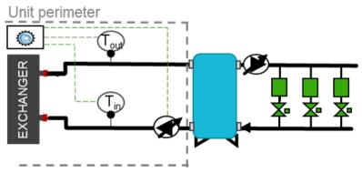
Flowzer VDT uses the temperature sensors installed at the inlet and outlet of the heat exchanger to automatically adjust the pump speed, thus keeping the T delta difference setpoint constant.
