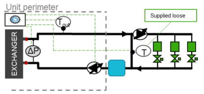
Bluethink solution for a variable flow rate system, consisting of a primary circuit plus secondary circuit. It is obligatory for the option to be combined with the Flowzer VP (inverter) and with one of the hydraulic modules that can be selected for the unit. The accessory is not compatible with Multilogic. Please contact our sales department for further details.
