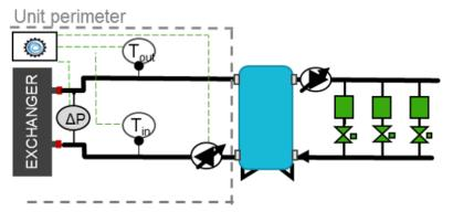
Bluethink solution for variable flow systems - ideal for systems featuring a primary and a secondary circuit physically divided by a heat exchanger or a tank with multiple connections. flowzer vps with TD-based control includes:
